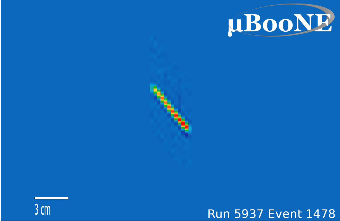
Figure 1: A proton candidate track in MicroBooNE data selected by a trained boosted decision tree. The wire spacing is 3mm. The pixel color is proportional to ionization charge density.
