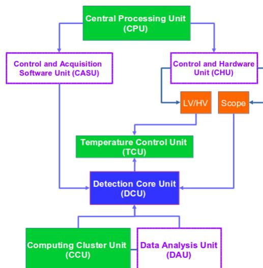
**Figure 1:** SiPMs and MPGDs characterization setup concept at UAN Detectors Laboratory.
