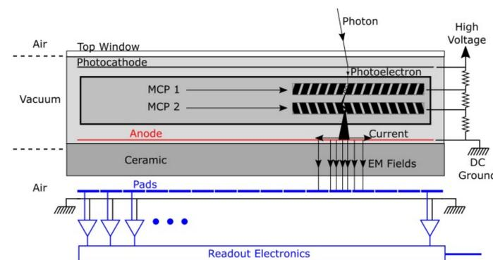
Figure 2: Micro-channel plates (MCPs) produce a shower of electrons, inducing fast signals on the anode. The signal is measured capacitively by a pickup outside.
