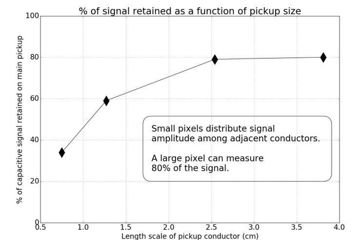
Figure 6: Small pixels will distribute pulse amplitude among neighboring channels. Pads larger than the signal spot size measures a maximum of 80% of the signal amplitude.
