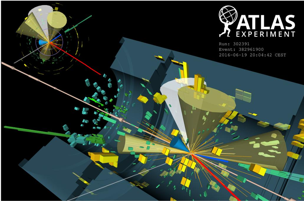
Figure 2: Event display of one of the candidate event in  $2\ell 1\tau_{\text{had}}$ . The blue track is the selected electron; the red track is the selected muon; the white cone is the  $\tau_{\text{had}}$  candidate; the three yellow cones are the selected jets and azure cone is the selected b-tagged jet. The green and yellow bars indicate the energy deposits in the electromagnetic and hadronic calorimeters [3].
