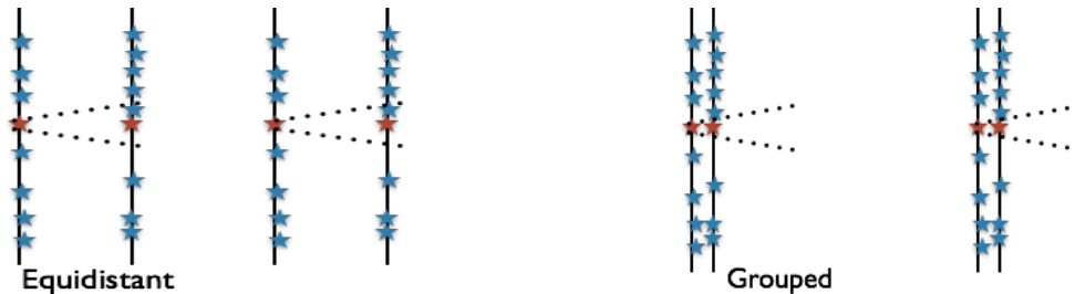
Figure 2: Illustration of segment building and linking in events with combinatorial background hits from pileup to contrast the equidistant layout (left) with the grouped layout (right). Segment building window, highlighted by dotted lines, is the same in both cases; it is defined by the acceptance needed for segment reconstruction. More combinatorial background hits are picked up in the equidistant layout and leads up in the equidistant layout and leads to more background segments.
