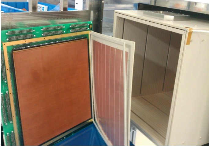
Figure 2: Interior view of the NEWAGE-0.3b' \mu -TPC. From the left: the \mu -PIC, the GEM, and the field cage.
