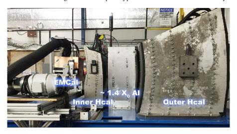
Figure 3: sPHENIX calorimeter prototypes in the FNAL test beam facility
