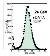
**Figure 5:** GEANT4 simulation and data comparison for 24GeV pion response
