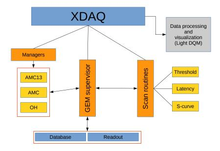
Figure 1: GE1/1 DAQ development structure.
