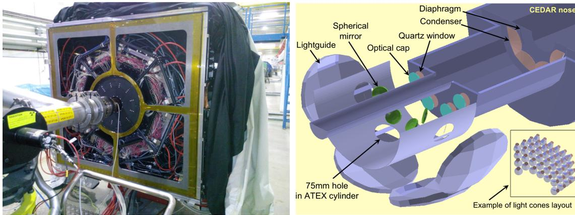
**Figure 2:** a) picture of the new KTAG detector positioned upstream the quartz windows, surrounding the nose and housing mirrors, light collection cones and PMTs; b) Screenshot taken from a Geant4 simulation of the KTAG. The components of the optical system outside the CEDAR vessel are sketched.
