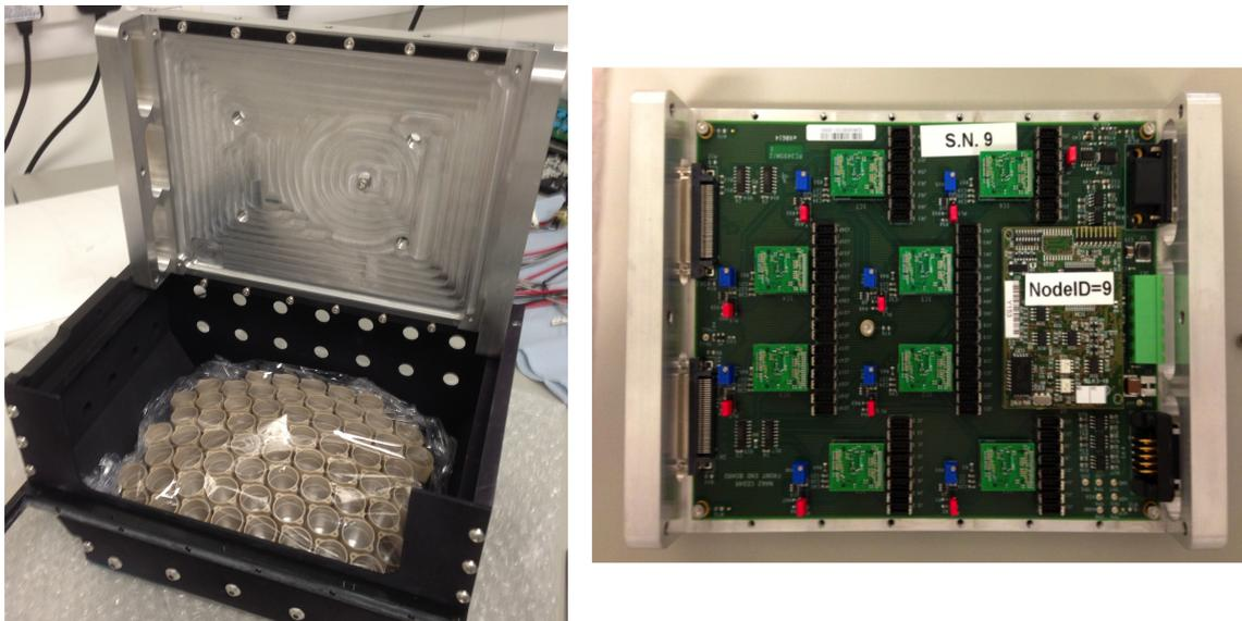
**Figure 3:** a) light box without PMTs, with the metallic lid lifted open and PMT holders attached at the basement. b) NINO board with two CAN bus connectors and a central voltage connector mounted at the right side of the board and two LVDS connectors at the left side of the board; the NINO board is screwed to the metallic lid of the light box.
