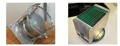
**Figure 1:** The upgraded light collection system with new PMTs (left) and the renovation of the read-out electronics with a compact lay-out (right) represent the most important tasks of the T600 overhauling.
