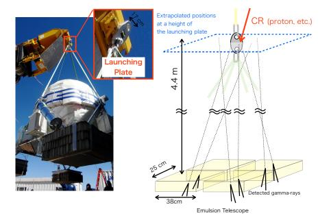
**Figure 2:** Left pictures show the gondola in GRAINE 2015 and the launching plate. Right schematic view shows the positional relation of the emulsion telescope and the launching plate. A square drawn with blue dotted lines indicates a plane at a height of the launching plate.
