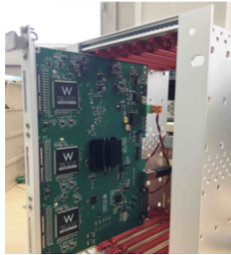
Figure 4: (Left) Schematic view of FEB layout. (Right) An image of the FEB in one of the racks.
