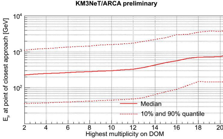
**Figure 3:** Expected muon energy at the point of closest approach to a DOM as a function of the multiplicity in single-muon MUPAGE MC events. If more than one coincidence occurs on the DOM in the event only the highest-multiplicity cluster is counted.
