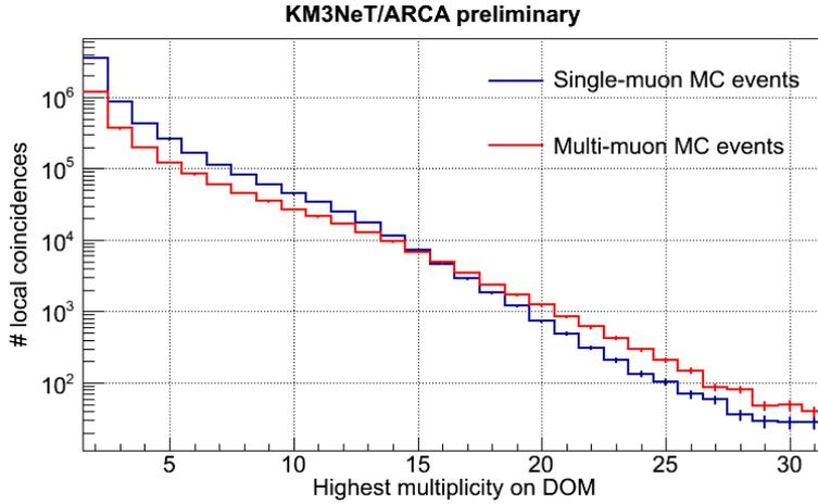
**Figure 1:** Distribution of the highest multiplicity induced on each DOM in atmospheric muon MC events. There is one entry per DOM with highest multiplicity  $\geq 2$  per simulated event. The contributions from single-muon and multi-muon MC events are shown separately.
