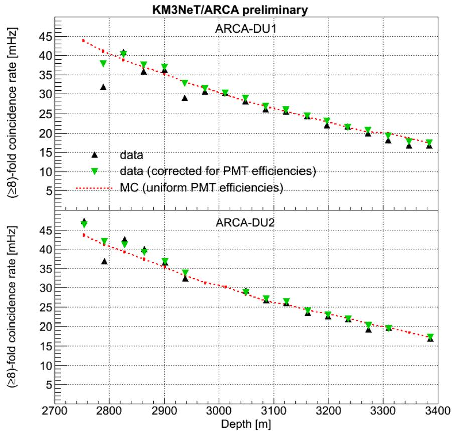
**Figure 5:**  $\geq 8$ -fold coincidence rate as a function of the depth below the sea surface. The red dashed line shows the base expectation from an ideal MC with uniform PMT efficiencies which neglects the differences between individual PMTs as determined from in-situ calibration. The black points show the uncorrected data. The green points show the data corrected for the effect of the PMT efficiencies. Statistical errors bars are included but are too small to be visible over the markers.
