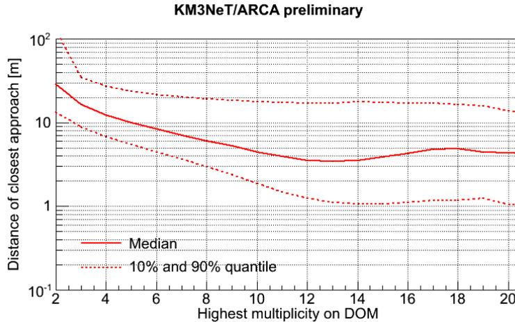
**Figure 2:** Distance of closest approach to a DOM as a function of the multiplicity in single-muon MUPAGE MC events. Muon tracks for which the expected track length does not reach up to the point of closest approach to the DOM are ignored. If more than one coincidence occurs on the DOM in the event only the highest-multiplicity cluster is counted.
