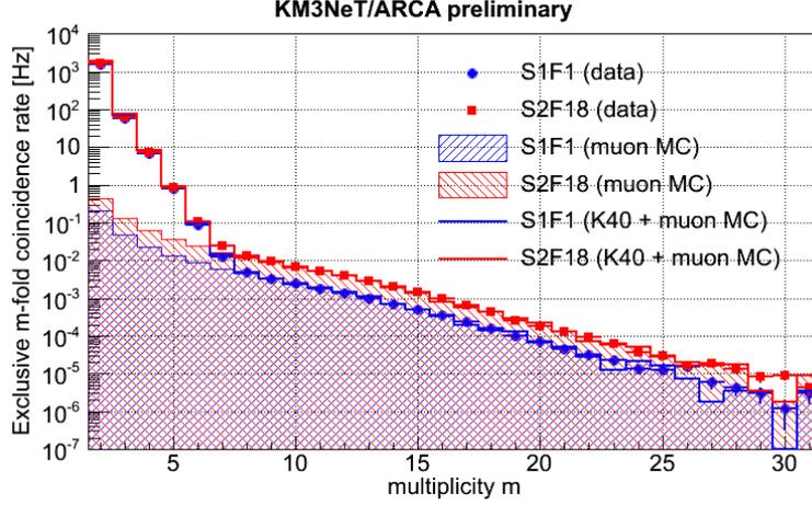
**Figure 4:** Coincidence rate as a function of the multiplicity. Two DOMs are shown: floor 1 (the lowest floor) of ARCA-DU1 and floor 18 (the highest floor) of ARCA-DU2. The data are overlaid with the expectations from MC simulations of  $^{40}\text{K}$  and atmospheric muons. Note that the PMT efficiencies in the  $^{40}\text{K}$  simulation have been varied within the systematic uncertainties in order to match the slope observed in data.
