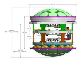
**Figure 4:** A drawing of the multi-PMT module hosting 3-inch PMTs. The upper (lower) hemisphere will cover the inner (outer) detector region.
