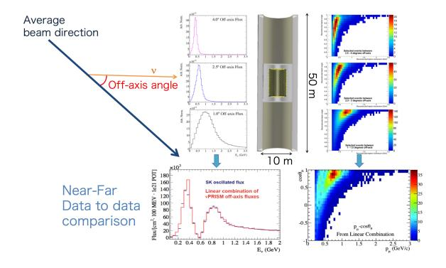
**Figure 3:** The use of a linear combination method in the E61 detector. A linear combination of off-axis fluxes is used to reproduce the oscillated flux at the far (here the Super-K) detector. Linear combination of different muon momentum and angle distributions predicts the muon kinematic distributions for the oscillated flux.
