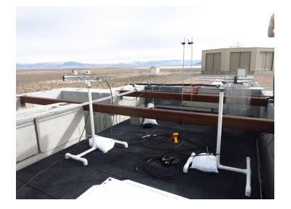
**Figure 2:** A front view of the LPDA set-up, consisting out of two EMCO LPDAs. During the experiment, the antennas were shielded by an RF absorbing screen.
