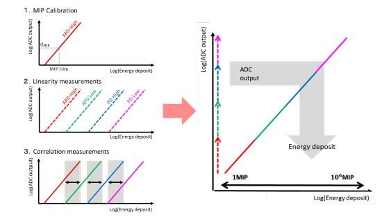
Figure 1: The conceptual diagram of the energy calibration processes.
