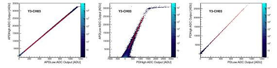
**Figure 4:** Typical gain correlation measurements between adjacent gain ranges. (*Left*) APD high gain to APD low gain, (*Middle*) APD low gain to PD high gain, and (*Right*) PD high gain to PD low gain regions.
