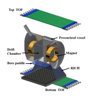
**Figure 1:** Partially sectioned 3D model of the High Energy Light Isotope eXperiment detector systems, showing superconducting magnet, drift chamber tracker, two time-of-flight layers and ring-imaging Cherenkov detector.
