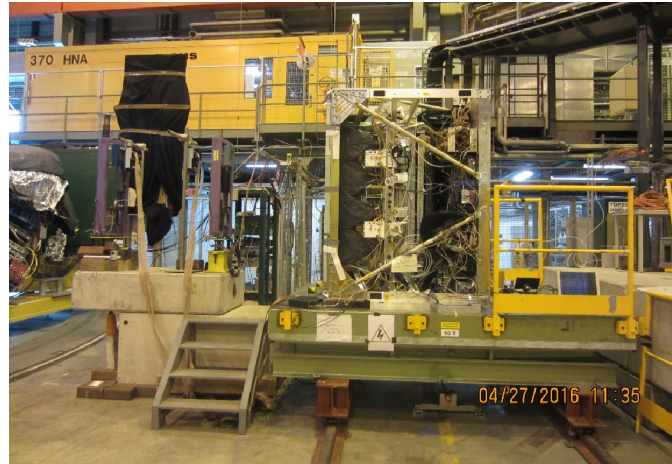
Figure 3: The BACCUS payload rotated by 90^\circ on a moving table in the H2 beam area at CERN.
