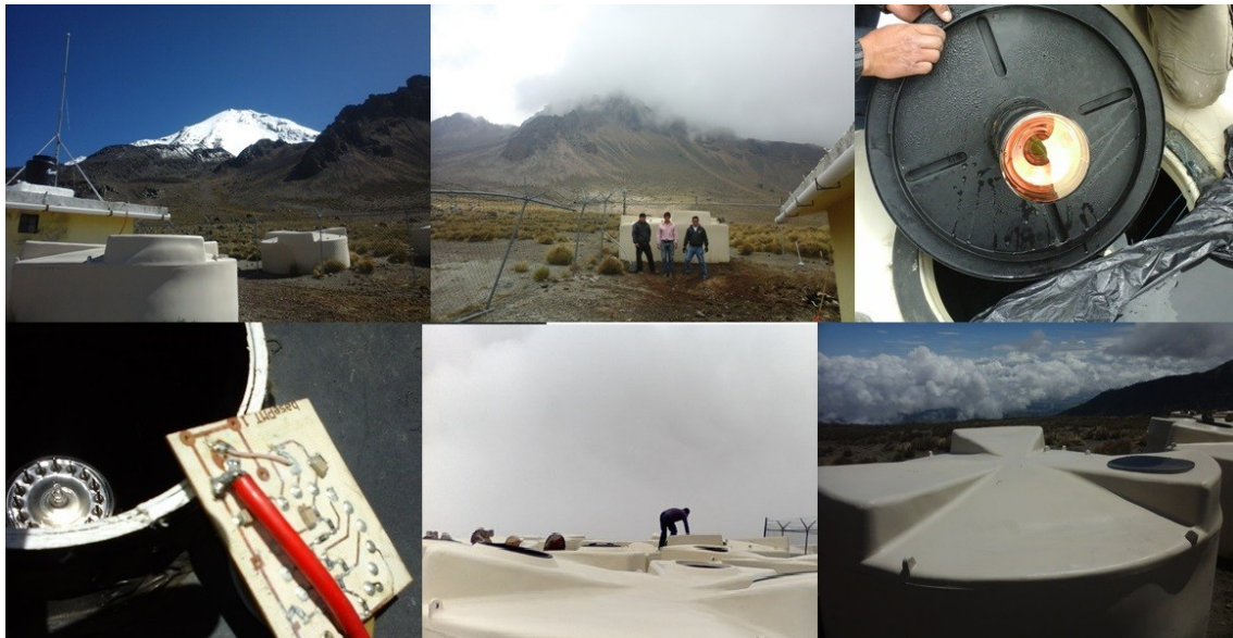
Fig.1 The CHARM Observatory site, located near at Pico de Orizaba Volcano at 4300m.a.s.l. In these pictures can see the tanks, eolic system of generating energy, the PMTs and electronic associated.
