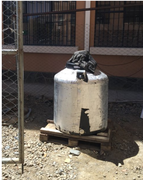
Figure 2: The prototype WCD situated at the university campus in Cota Cota. The PMT case can be seen at the top of the tank.
