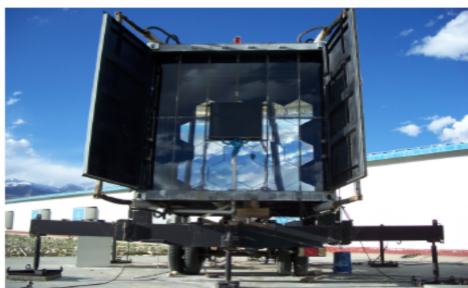
Figure 1: WFCTA prototype, including a reflecting mirror and a 256 PMTs array
