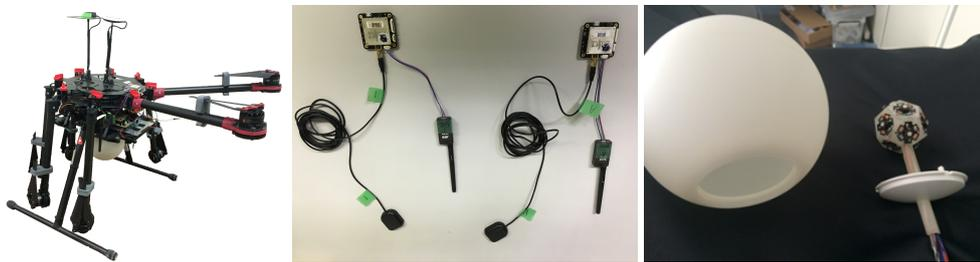
**Figure 2:** (Left) The eight rotor multicopter (S1000+, DJI) mounting the LED flasher under the body. The arms can be folded. (Middle) High accuracy GPS. One is installed at the well known point as base and the other is mounted on Opt-copter. (Right) UV-LEDs installed on the dodecahedron which will be covered by the spherical diffuser.
