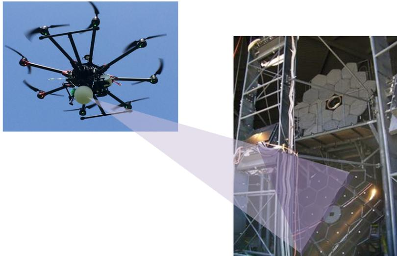
**Figure 1:** The diagram of FD calibration concept using Opt-copter. UAV with a LED light flasher is flying to the F.O.V. of TA FD.
