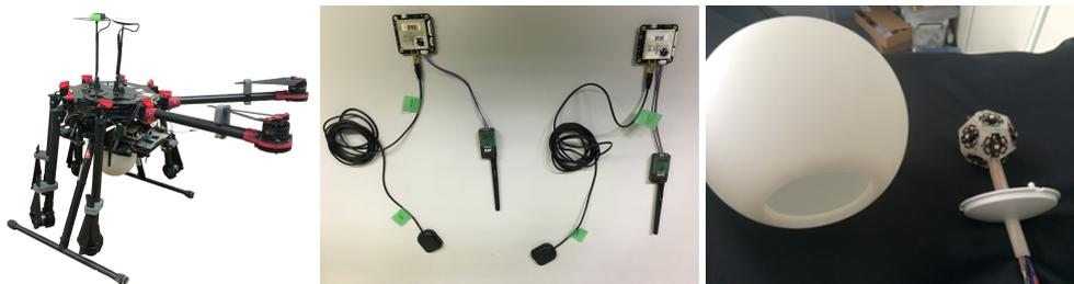
**Figure 2:** (Left) The eight rotor multicopter (S1000+, DJI) mounting the LED flasher under the body. The arms can be folded. (Middle) High accuracy GPS. One is installed at the well known point as base and the other is mounted on Opt-copter. (Right) UV-LEDs installed on the dodecahedron which will be covered by the spherical diffuser.
