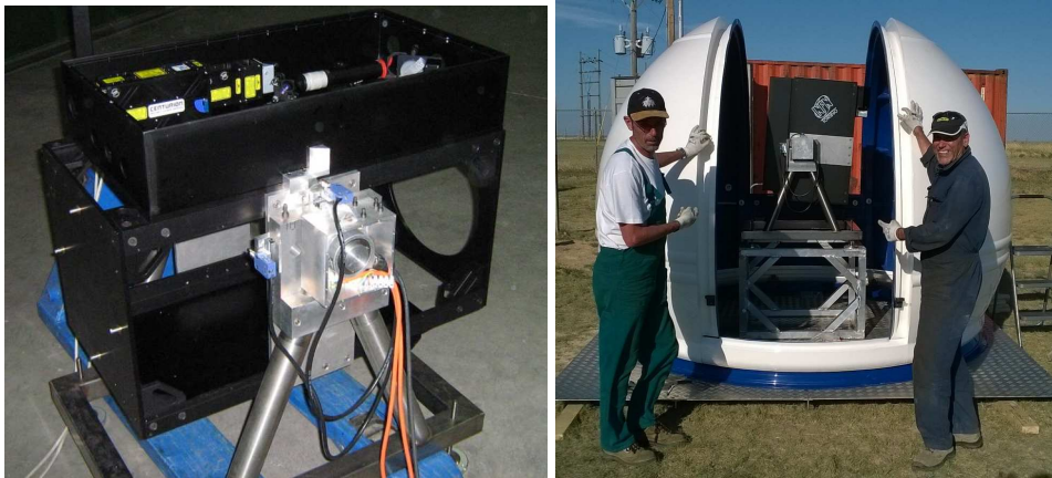
Figure 2: On the left, the ARCADE telescope. On the right, the dome with the telescope installed within.
