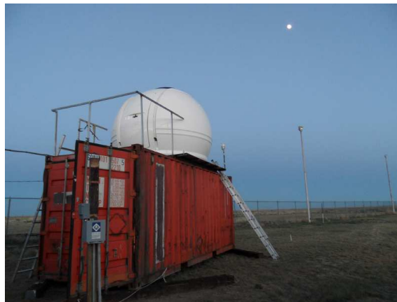
Figure 3: The astronomical dome containing the Lidar, on top of the 20 ft shipping container used in Lamar, Colorado
