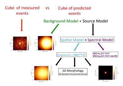
**Figure 1:** Illustration of the construction of the cube of predicted events for one energy band from the background cube, the exposure and PSF cube. The spectral and spatial parameters are then fitted by comparing the predicted cube events to the measured cube events for each pixel of the images and each energy bin of the cube.
