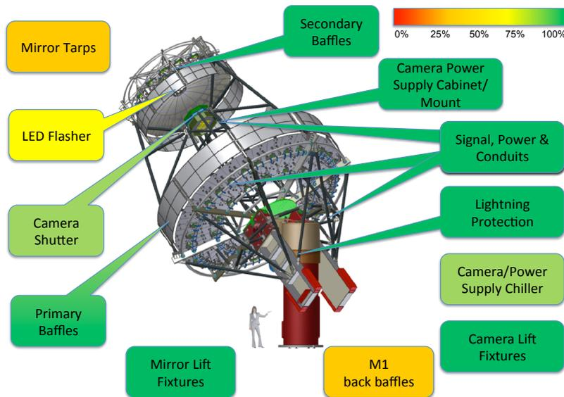
Figure 3: Completion Status of pSCT Auxiliary Equipment.
