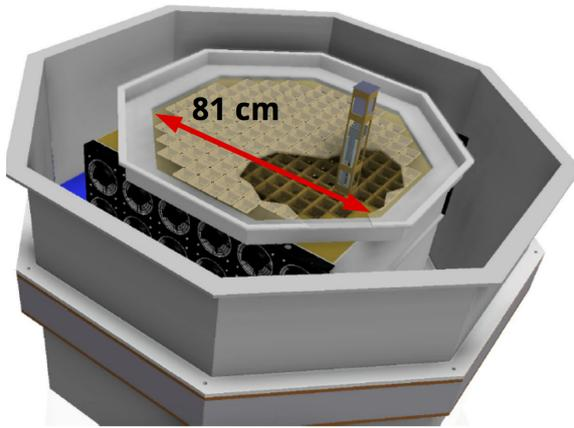
Figure 5: pSCT camera hierarchical concept. One of 177 FEE modules is pulled up and shown.
