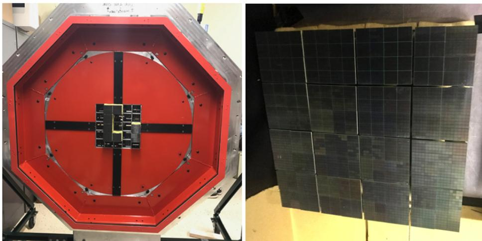
Figure 6: Assembled mechanical structure of the camera (*Left*). Eight FEE modules installed into pSCT camera (*Right*).
