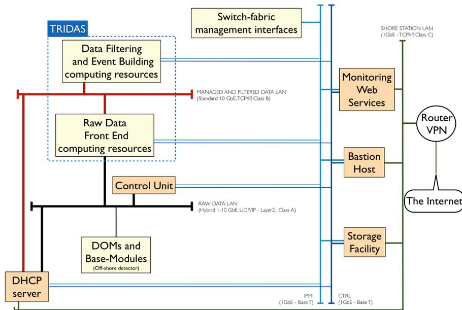
**Figure 1:** The KM3NeT network segments with the basic elements of the Trigger and Data Acquisition System and the other computing resources available at the shore-stations. See text for details.
