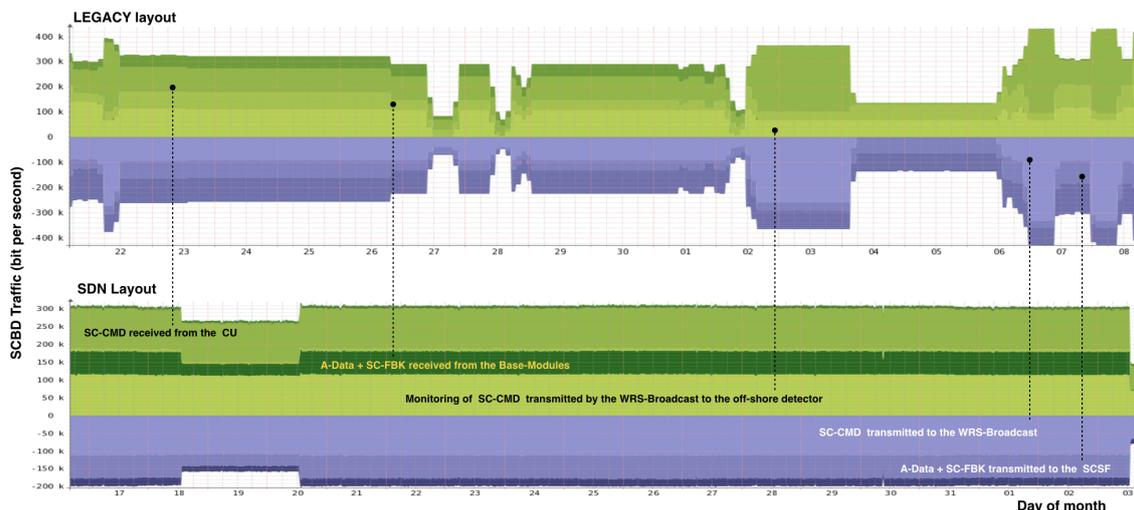
**Figure 3:** The comparison of the traffic through the SCBD during two different data-taking periods: top, with the Legacy layout; bottom: exploiting the SDN layout. Diagrams with shades of green and violet stand for incoming and outgoing throughputs in the SCBD, respectively.
