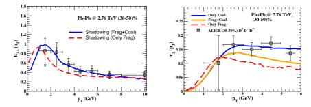
**Figure 1:** Left and middle panel: D meson  $R_{AA}$  and  $v_2$  respectively in Pb + Pb collisions at  $\sqrt{s} = 2.76$  ATev and centrality 30 - 50% compared to ALICE data. Experimental data has been taken from Ref.s [15, 16].
