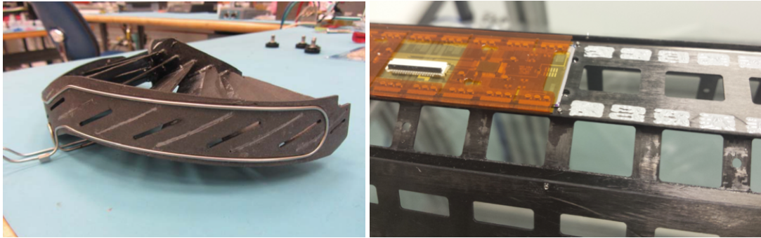
Figure 2: CO 2 cooling tube embedded in FPIX disk (left). Cooling lines between the BPIX ladder (right) [5].
