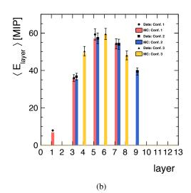
Figure 3: Average energy deposited in the detector planes as a function of the number of absorber layers for three configurations combined (a) and separately (b). The dots are data and the shaded area corresponds to the MC simulation.
