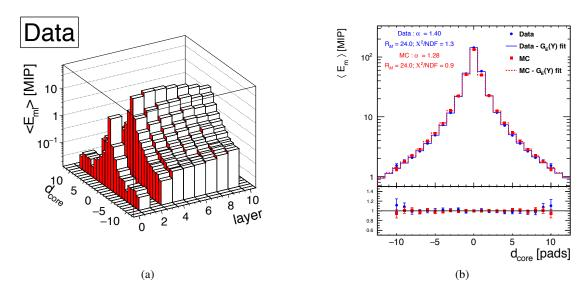
Figure 5: (a) A lego plot of  $\langle E_{ml} \rangle$ , as a function of  $d_{core}$  in units of pads, for each layer from the beam test data. (b) The shower transverse profile  $\langle E_m \rangle$ , as a function of  $d_{core}$  in units of pads, of the sum of all three configurations from beam test data and the MC simulation, after symmetry corrections and fit. For the data (blue) and the MC (red).
