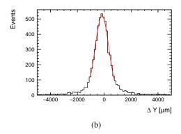
Figure 4: (a) The deposited energy sum for a single event,  $E_n$ , as a function of Y expressed in terms of the pad number. The curve is a Gaussian fit to the data. (b) The distribution of the residuals between the reconstructed positions,  $\Delta Y$ . The curve represents the Gaussian fit to the distribution
