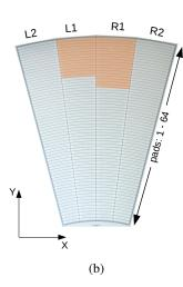
Figure 1: (a) The very forward region of the ILD detector. (b) A LumiCal prototype silicon sensor. The shaded area denotes the pads that were connected in this test.
