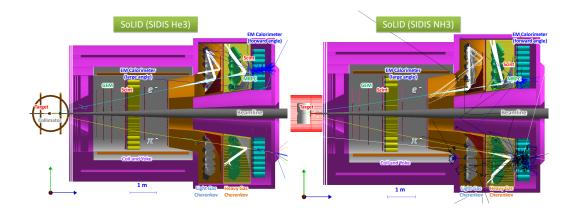
**Figure 1:** The experimental layout of the SoLID SIDIS setup with the  ${}^{3}$ He (left) or NH<sub>3</sub> (right) target. The scattered electrons are detected by both forward-angle and large-angle detectors. The leading pions are detected by the forward-angle detector only.
