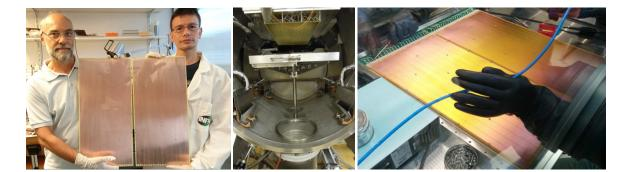
**Figure 3:** Two THGEMs before the post-production treatment (left), a THGEM inside the CsI evaporation plant (center), THGEMs being mounted on a COMMPASS Hybrid PD inside a glove-box (right).
