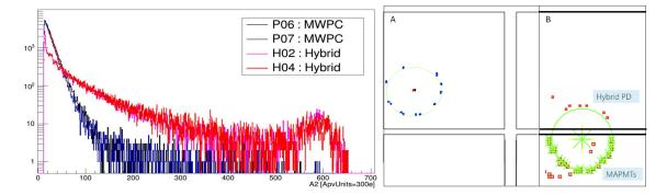
**Figure 4:** Signal amplitude distributions for MWPCs and Hybrids (left). Two Cherenkov rings from a typcal RICH-1 event in COMPASS 2017 data taking (right).
