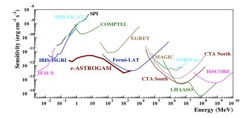
Figure 3: Point source continuum sensitivity of different X and  $\gamma$ -ray instruments compared with e-ASTROGAM.
