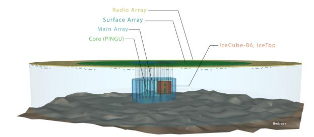
**Figure 1:** Schematic drawing of the IceCube-Gen2 facility including the main array, a densely instrumented core, a large surface and a radio array. This document focuses on the main array and surface array.
