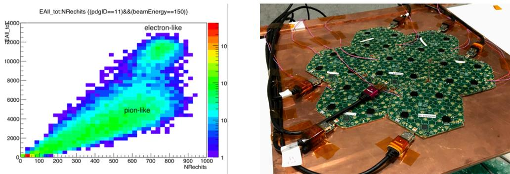
**Figure 3:** *Left:* total deposited energy plotted against the total number of hits in the prototype for a run with 150 GeV electrons and a strong pion contamination corresponding to the lower population. *Right:* seven 6" silicon sensor modules mounted on a copper support & cooling plane during the 2017 beam test campaign.
