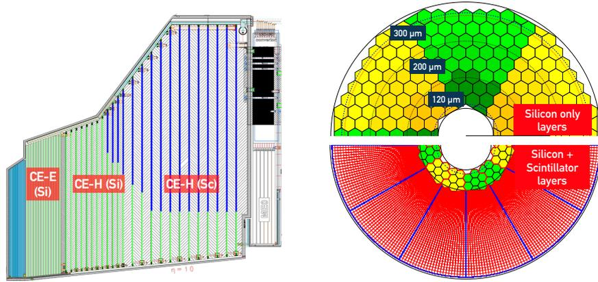
**Figure 1:** *Left:* Transverse illustration of the HGICAL highlighting the silicon and scintillator compartments in green and blue, respectively. *Right:* layout of a silicon-only (top) and mixed silicon-scintillator (bottom, not to scale) layer indicating the different silicon wafer thickness regions.
