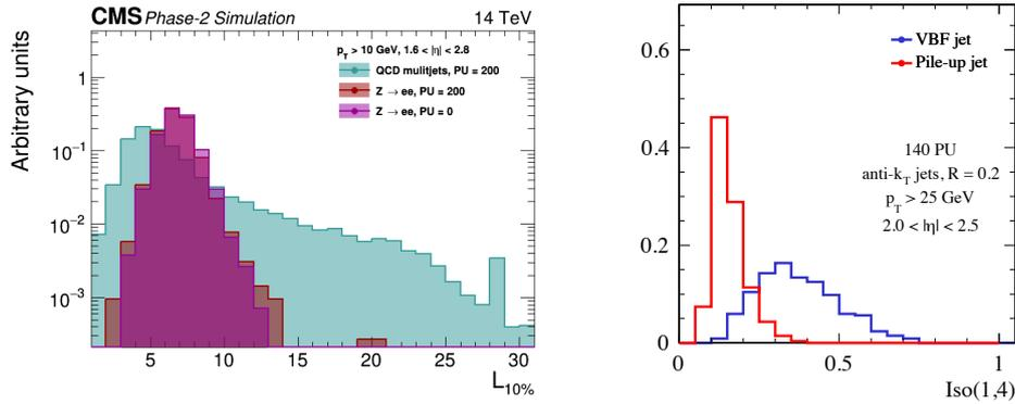
**Figure 2:** *Left:* distributions of the layer number at which the cumulative longitudinal energy exceeds 10% of the total energy in a cluster for true electron clusters with and without pileup to clusters from QCD multijet showers. *Right:* comparison of the relative isolation for pileup jets and jets from VBF production.
