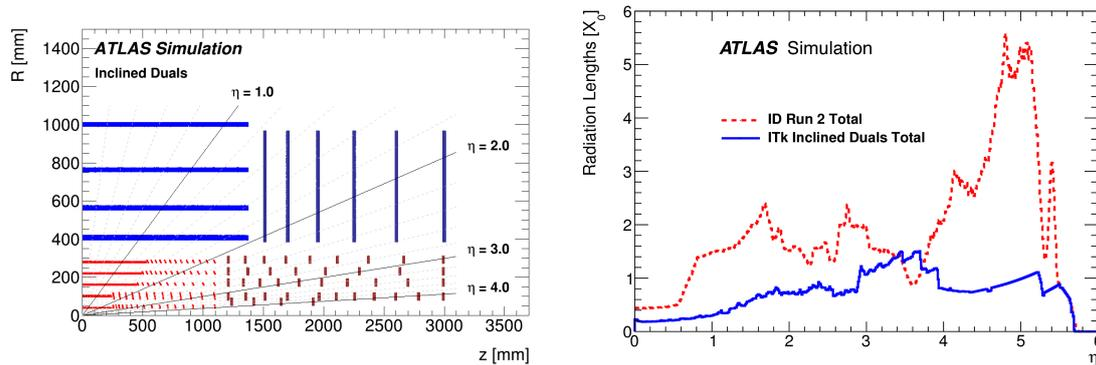
Figure 1: **Left:** Schematic view of the Inclined Duals layout showing the sensors position in one quadrant of the  $(r, z)$ -plane. Pixel (Strip) sensors are shown in red (blue) [2]. **Right:** Comparison of ID (red dashed line) and ITk (blue solid line) material budget in terms of  $X_0$  versus  $\eta$  [2].
