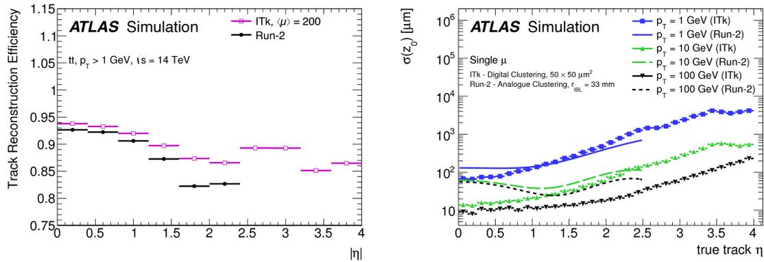
Figure 2: **Left:** Track reconstruction efficiency of the ITk for a top-pair sample with an average of 200 pile-up events. Results for the current ID with a Run2-like pile-up distribution are also shown [2]. **Right:** Track  $z_0$  resolution versus  $\eta$  for  $50 \times 50 \mu\text{m}^2$  pixels. Results are shown for single muons of 1, 10, and 100 GeV in  $p_T$ . The resolutions for the current ID are overlaid [2].
