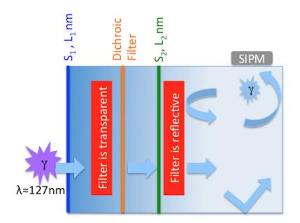
**Figure 2:** Demonstration of an Arapcua. UV photons are able to penetrate the second filter, denotated by the green line, but are unable to exit, resulting in visible photons being "trapped" in a reflective box. The trapped photons are eventually detected by arrays of SiPMs, shown on the top.
