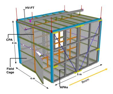
**Figure 1:** Three-dimensional model of the short baseline near detector TPC. The two drift regions are realized with two anode plane assemblies (APA), and one cathode plane assembly (CPA) in the center of the TPC.
