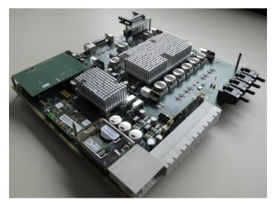
Figure 1: L1Topo Module during Run-2. The FPGAs are covered by heat sinks.
