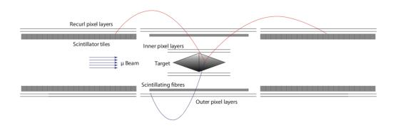
Figure 4: Experimental setup of the Mu3e experiment.
