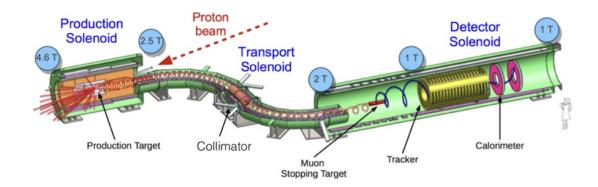
Figure 3: Experimental setup of the Mu2e experiment.
