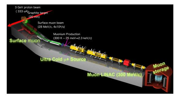
Figure 5: Experimental setup of the J-PARC muon g-2/EDM experiment.
