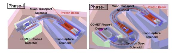
Figure 2: Schematic view of the COMET experiment setups for Phase I (left) and Phase II (right)
