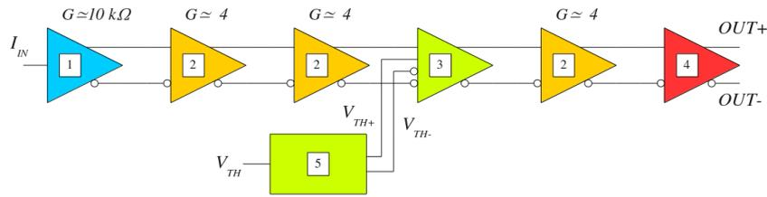
**Figure 3:** TIA-based architecture
