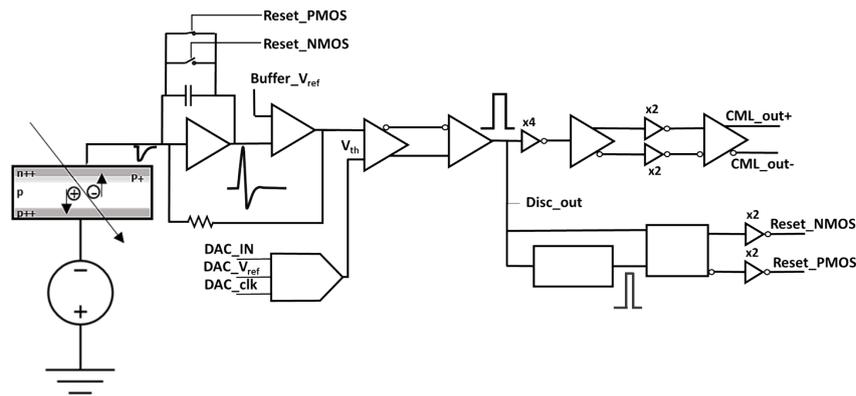
Figure 2: CSA-based architecture
