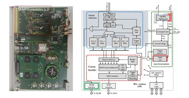
**Figure 1:** On the left a picture of the Digitizer Board fully equipped. A second mezzanine is present at the bottom of the board, hosting the TDC chips used in the PPS project. On the right a scheme of the readout section of the firmware developed for the SF2 FPGA.
