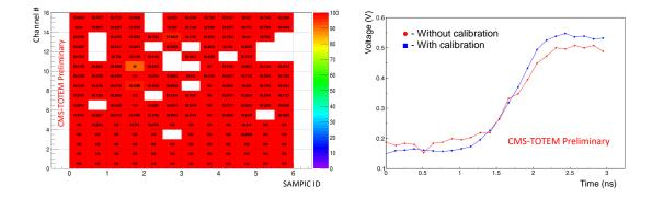
**Figure 2:** On the left the transmission efficiency for all the channels. On the right an example of waveform, before and after the offline calibration procedure.
