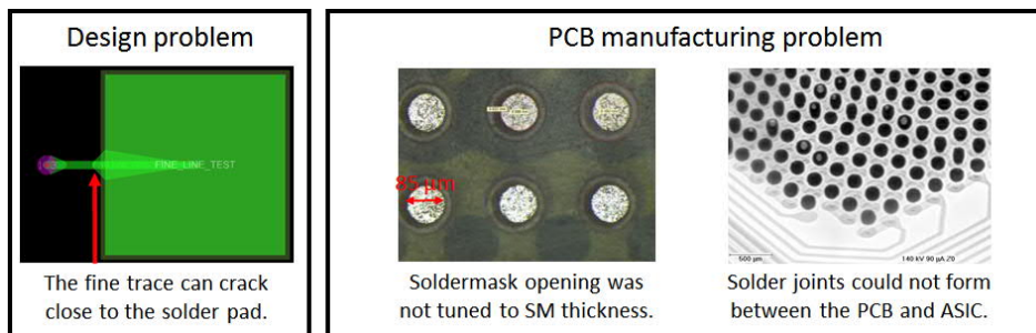
Figure 5: Other failures caused by design and PCB manufacturing problems.
