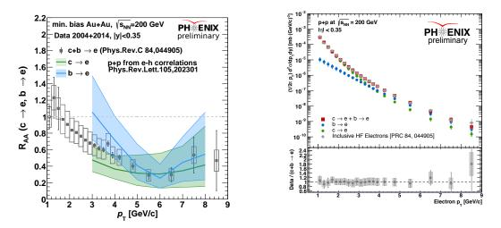
**Figure 4:** (a, left)  $R_{AA}$  for inclusive electrons from charm and bottom quarks, and electrons from charm and bottom quarks separately, measured in minimum bias Au+Au collisions at  $\sqrt{s_{NN}} = 200$  GeV. (b, right) New p+p baseline of the electrons from charm and bottom quarks.
