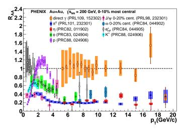
Figure 1: Latest compilation of  $R_{AA}$  for various particles in 0-10 % Au+Au collisions at  $\sqrt{s_{NN}} = 200 \text{ GeV}$ .
