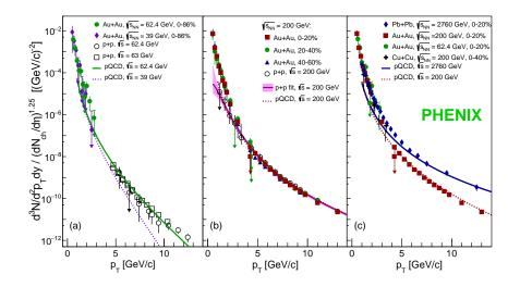
**Figure 6:** Direct photon invariant yields scaled by  $(dN_{ch}/d\eta)^{1.25}$  for (a, left) Au+Au collisions at 39 and 62.4 GeV together with p+p and pQCD calculation, (b, middle) Au+Au collisions at 200 GeV for several centralities, and (c, right) central Au+Au, Cu+Cu and Pb+Pb collisions.
