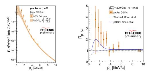
**Figure 7:** (a, left) Direct photon spectra in 0-5 % *p*+Au collisions at  $\sqrt{s_{NN}} = 200 \text{ GeV}$  together with the parameterized *p*+*p* yield scaled by  $N_{\text{coll}}$ . (b, right)  $R_{\text{pA}}$  of the direct photons.
