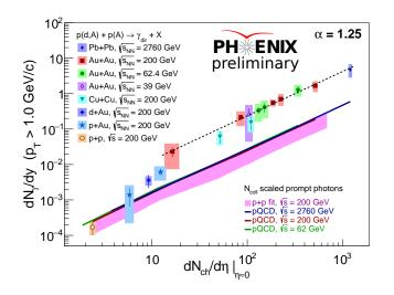
**Figure 8:** Integrated photon yield  $(p_T > 1 \text{ GeV}/c)$  as a function of  $dN_{ch}/d\eta$  for various collision systems.
