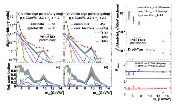
**Figure 9:** (a, left) Invariant mass spectra for muon-pairs in forward and backward rapidities in *p*+Au collisions at  $\sqrt{s_{NN}} = 200$  GeV, together with the various known hadron contributions. (b, right)  $p_T$  spectra for the extracted Drell-Yan contribution for *p*+*p* (scaled by  $N_{coll}$ ) and *p*+Au collisions, and corresponding  $R_{pA}$ .
