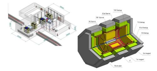
Figure 10. Composition of the SPD setup at parking position in experimental building and at the collider beam line
