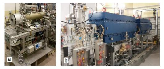
**Figure 6.** Special ion source prepared for heavy ion run at linac LU-20 and Nuclotron for the BM&N setup data taken (a) and the new linear accelerator HILAC for NICA heavy ion injection chain (b).
