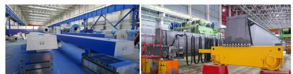
**Figure 9.** Manufactured 25 from 28 of yoke plates: 0.35x0.74x8.47, m3; 16 tons each are ready (left part). Two 80 ton cranes for the MPD and SPD halls were prepared and tested (right part).
