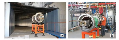
Figure 2. The "tunnel" with the Nuclotron magnet block (a) and the booster dipole magnet at test bench (b).
