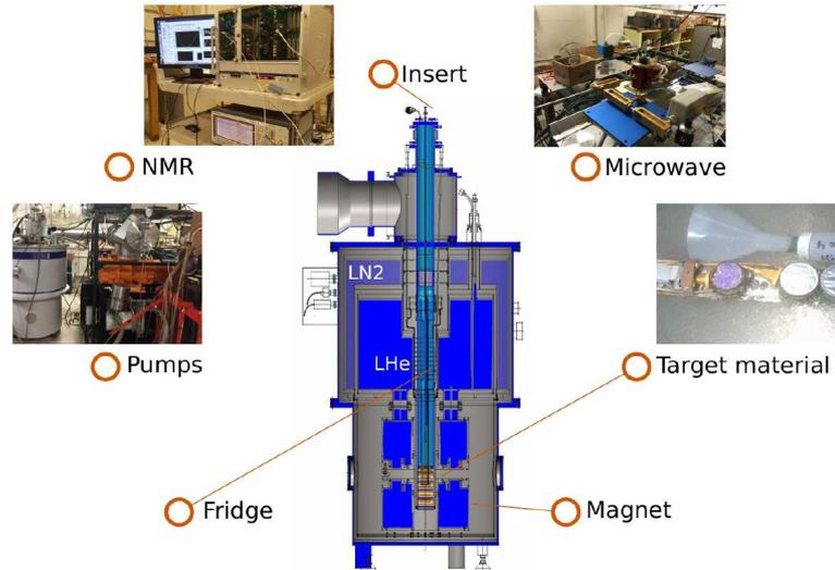
**Figure 7:** The target system of SpinQuest shown together with its supporting devices.
