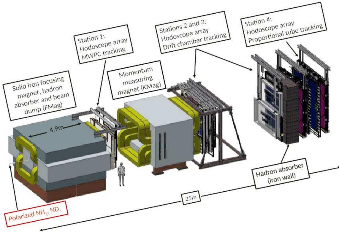
**Figure 6:** The spectrometer of the SeaQuest/E906 is used in SpinQuest experiment.
