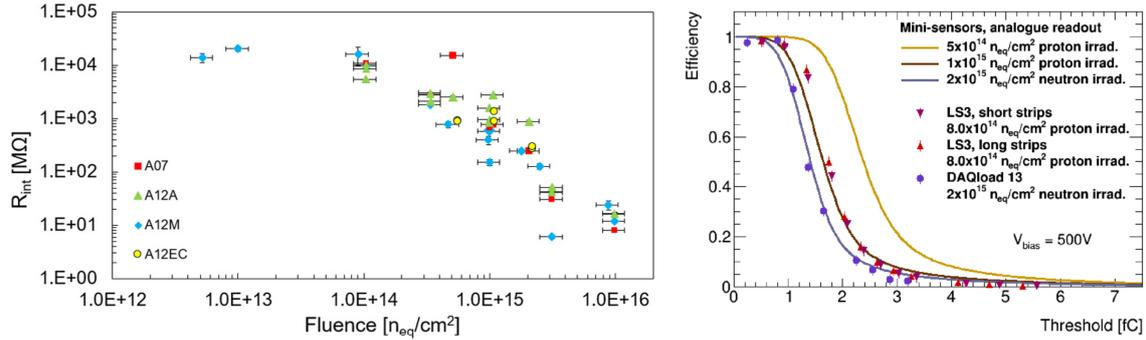
**Figure 3:** Left: Interstrip resistance evolution with irradiation with protons on different sensor prototypes at a depletion voltage of 400 V [7]. Right: Comparison of threshold scans of differently irradiated module prototypes [2].
