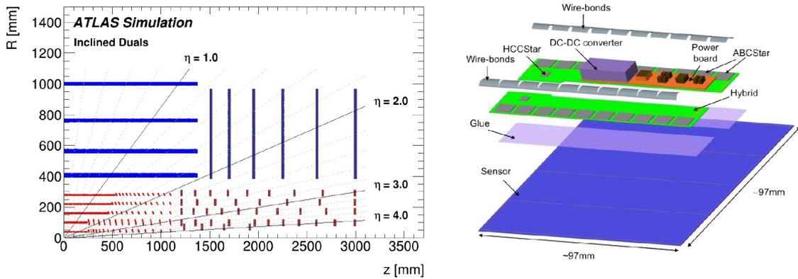
**Figure 1:** Left: The Schematic layout of the ATLAS ITk detection layers shows their placement in the cylindrical coordinate system [3]. Right: Assembly schema of a short strip barrel module [2].
