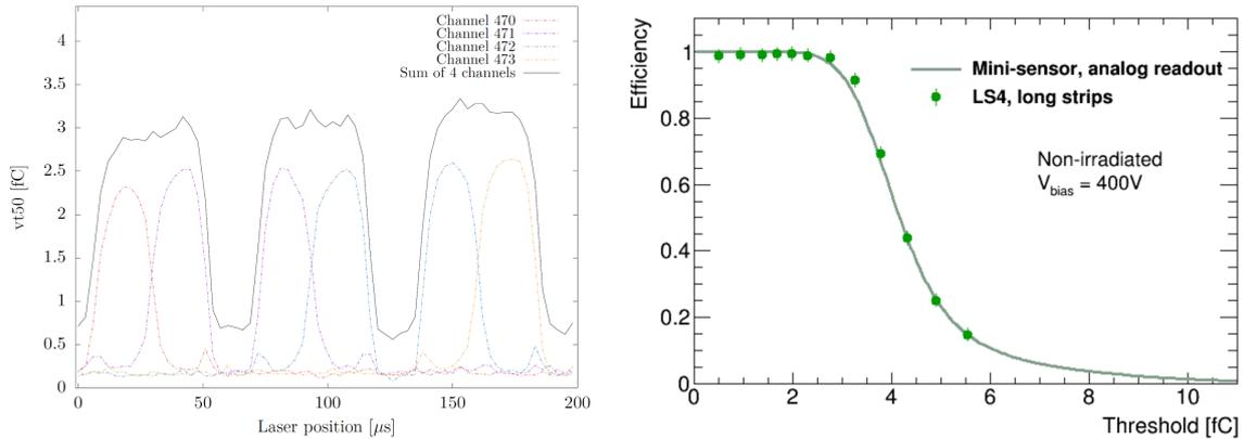
**Figure 2:** Left: A laser interstrip scan of an ITk strip miniature sensor [4]. Right: Comparison of CERN test beam results reconstructed in the low-cluster-size region (dots) and sensor charge collection studies done with the  $^{90}\text{Sr}$  source and analogue readout (line) [2].
