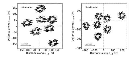
**Figure 1:** LOFAR antenna's are grouped into circular stations. Each antenna's polarization direction is shown with a black arrow. The y-axis represents the direction of  $(v \times v \times B)$  and the x-axis is the direction of  $(v \times B)$ . The left plot is the expected polarization direction for a "normal" fair-weather air shower. The right plot shows that the cosmic ray shower shows a different polarization than expected due to the thunderstorm.
