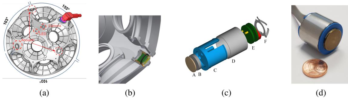
**Figure 3:** Acoustic sensor design. The figures show from left to right (a) possible positions within the mDOM’s holding structure (b) mounting concept for the sensor in the holding structure (c) exploded view of the sensor and its components (d) picture of an assembled prototype sensor
