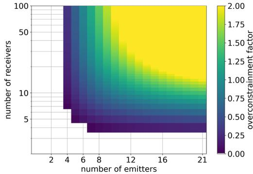
**Figure 2:** Overconstraint factor  $O$  as function of the number of emitting pingers and receiving mDOMs. Note, that the plot is clipped at zero and white regions correspond to underconstrained combinations. For larger values of receivers and emitters the boundaries remain straight.
