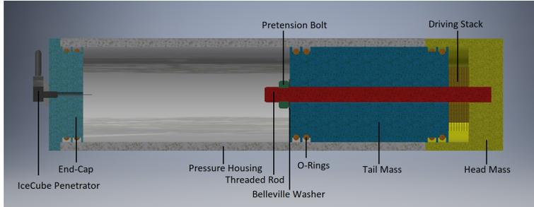
**Figure 4:** Design of the emitting pinger unit
