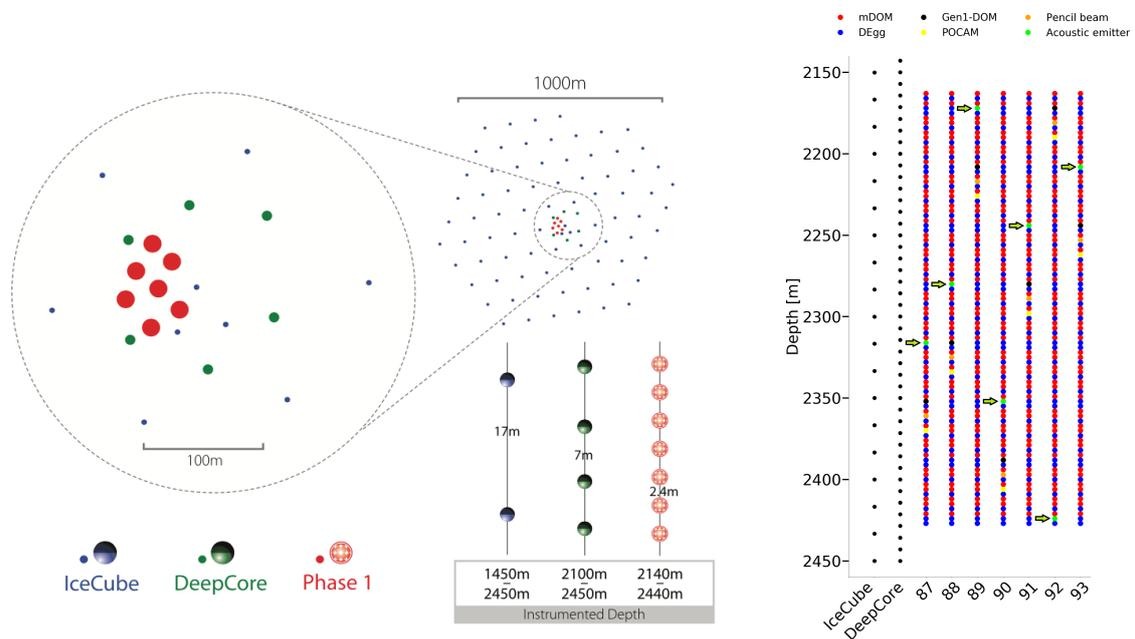
**Figure 1:** Geometry of the IceCube upgrade. The left figure shows the footprint of the new strings within the IceCube detector. The densely instrumented region (physics region) between depths of 2140 m to 2440 m is shown right with the positions of the acoustic pingers marked.
