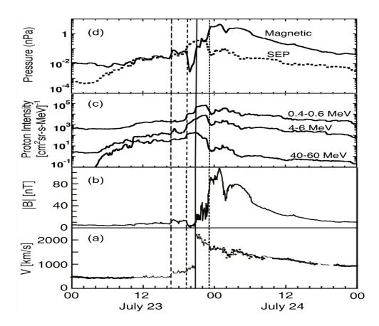
**Figure 5:** Time history of the July 23, 2012 event observed by STEREO-A (see [5]. This 4-panel Figure shows details of the July 23, shock that resulted in a very intense ESP event. Panel A (bottom) shows the solar wind speed, which reached 2280 km/s. Shortly threreafter the magnetic field reached 108 nT,.
