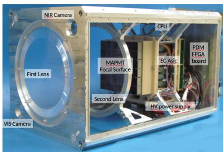
**Figure 4:** Telescope mechanical body with subsystems.
