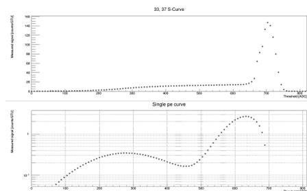
**Figure 11:** Top: Single pixel S-curve showing counts over a discriminated ADC threshold value. Bottom: S-curve derivative. The threshold for the single photoelectron is placed in the plateau between the left peak and the right pedestal (between 400 and 500 ADC).
