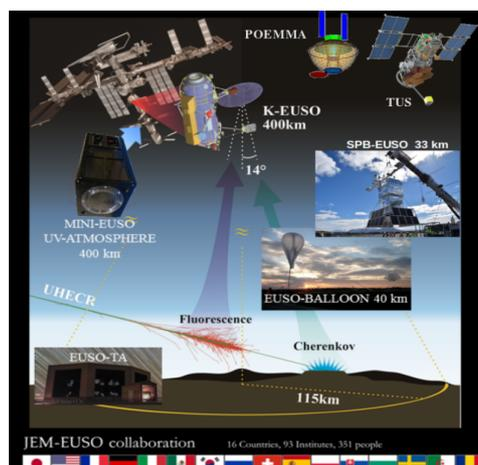
**Figure 1:** Roadmap of the EUSO telescopes: a) EUSO-TA: Ground detector installed in 2013 at Telescope Array site, with focal surface installed in 2015. b) EUSO-Balloon: 1st balloon flight from Timmins, CA (French Space Agency) August 2014; c) NASA Super Pressure Balloon (SPB) flight:2017; d) TUS on Lomonosov satellite, 2016; e) MINI-EUSO (2019) inside of International Space Station (ISS); f) K-EUSO [8]; g) POEMMA [9]
