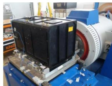
**Figure 10:** Mini-EUSO accomodation on the shaker - X direction
