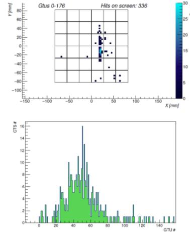
**Figure 3:** Top: UV Photon counts observed in the Mini-EUSO focal surface for a simulation of an  $E = 1 \times 10^{21}$  eV with an inclination of  $80^\circ$  to the nadir. Bottom: Light curve for the same event as a function of time in units of GTU (1 GTU =  $2.5\mu s$ ). [11]
