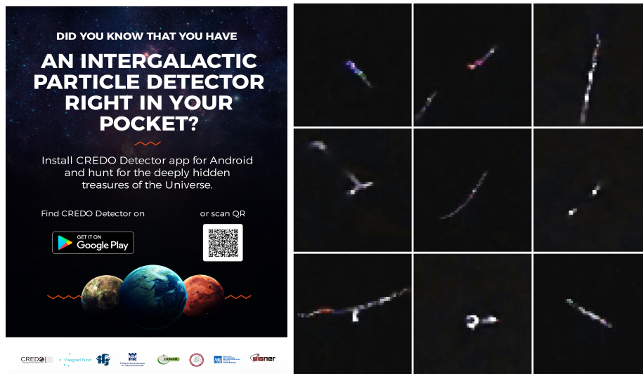
Figure 2: Left panel: The CREDO Detector app on Google Play; Right panel: Tracks of particles detected by the CREDO Detector app.
